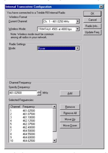
To reduce battery consumption on your base receiver, set the wireless mode as high as possible. For example, 9600 bits per second (bps) consumes half the power of 4800 bps for the same data format and time of operation.
