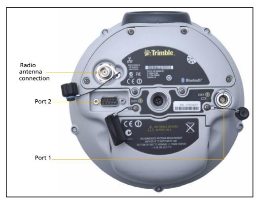
Each port or connector on the receiver is marked with an icon to indicate its main function as shown below.
